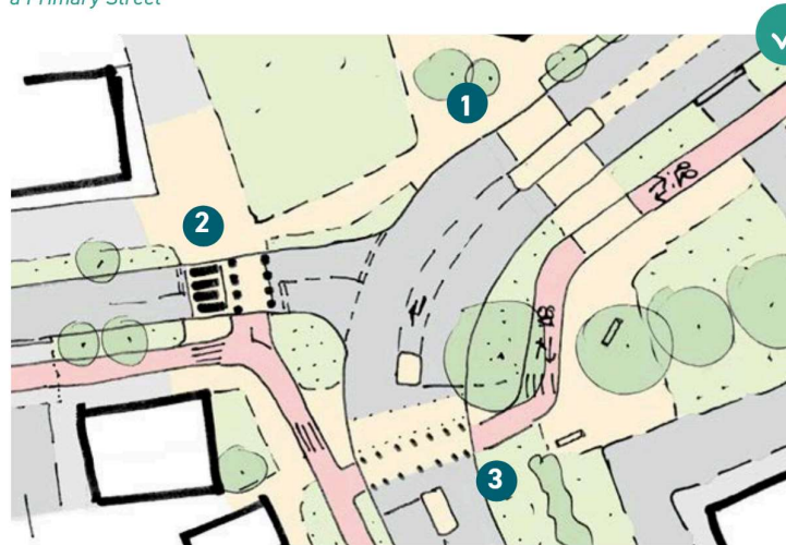
Illustrative layout of an informal crossing (1), a parallel crossing (2) and a toucan crossing (3)
